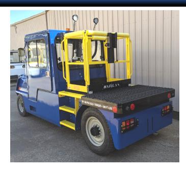
Designed as a multi-purpose vehicle for airside maintenance. The rear bed can be customized to fit your maintenance needs and its versatility lends itself for baggage/cargo applications.
